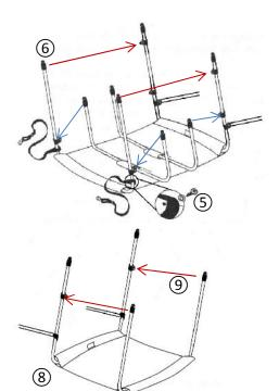
The following diagram is important to help you mount the bimini tops in the most desirable and functional position. All measurements provided are on-center of all deck hinges and eye straps. Pencil all locations before attempting installation so that changes can be made if desired. Since the locations of side gates can vary by boat brand and model, adjustments may be necessary to avoid side gates when mounting the bimini tops.
