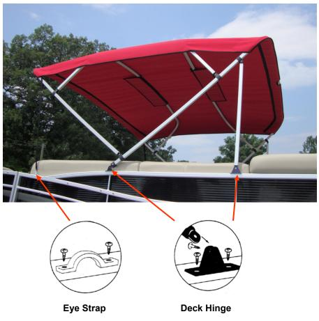
Important note to Top Installer/User: Be sure all set screws, fittings and pre-installed hardware are tight. Vibration can cause screws to loosen over time. Check all fittings frequently and tighten as necessary.
