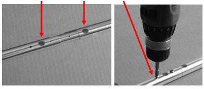
Step 3. Repeat this procedure for the medium (B-bow) and short (C-bow) , aligning the pre-drilled holes and securing them with  $#8 \ge 1/2$ " screws.
