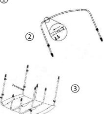
Begin assembly with the main 4-bow bimini top. These instructions show how to assemble the top, with its frame and straps, starting upside-down and inverting to an upright position when attaching to your boat.
