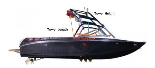
Fits boats with the tower mounted over the windshield with the top of the tower not to exceed 24" behind the wing of the windshield. Max tower height from top of gunnel: 68". See diagram. Wakeboard racks must be folded in and bimini tops must be folded down in order for cover to fit.
