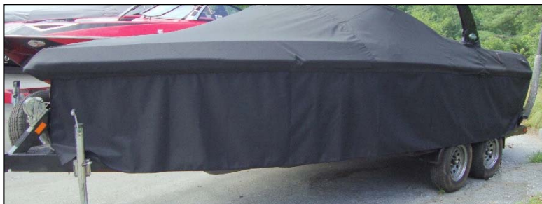
Installed Boat Skirt
