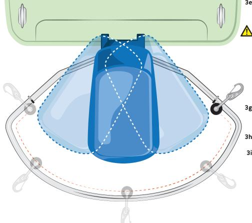
**3e.** Slide the pulley left and right to be sure that it cannot hit any part of the motor.
