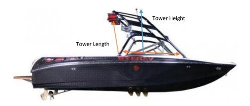
Fits boats with the tower mounted over the windshield with the top of the tower not to exceed 24" behind the wing of the windshield. Max tower height from top of gunnel: 68". See diagram.
