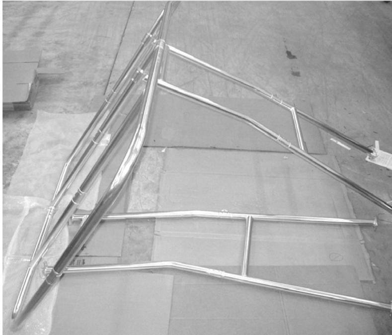
**Move the T-Top to the Boat:** It is easiest to have two people on the ground transfer the T-Top in the vertical position to two people in the boat. With only two people one can lift the canopy frame and the second can lift at the base of the legs to transfer to the boat in the horizontal position with one leg on the side of the boat. The key is to take it slow to prevent damage to the boat or T-Top.
