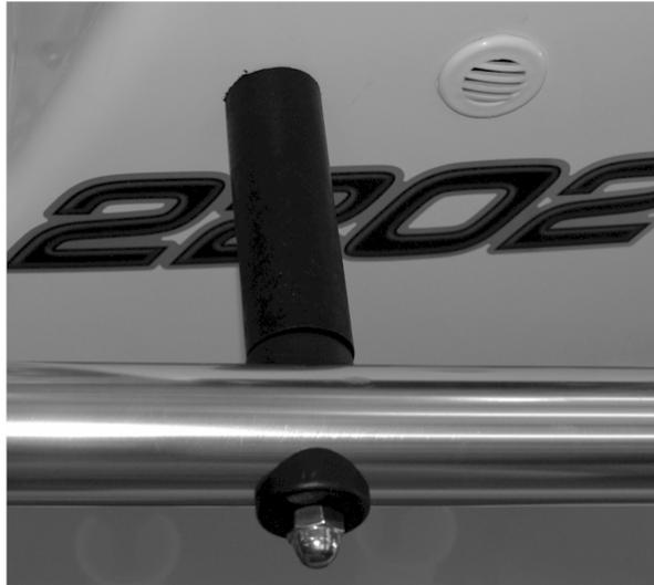
Complete the first standoff installation using Loctite tightening both the Acorn Nut and Backing Plate Nut.
