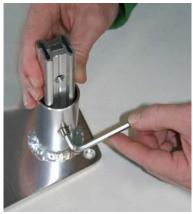
2. Next insert the tube connectors into the grab bar and loosely insert set screw into each hole. Once the legs are lined up properly tighten all the set screws.
