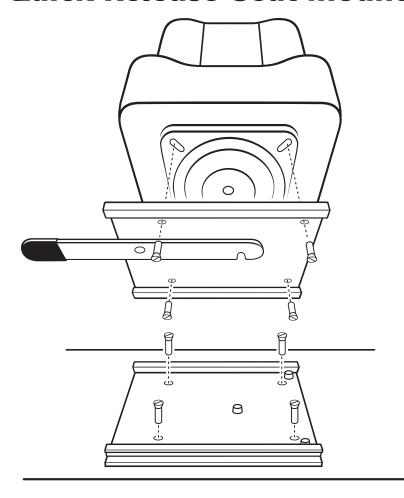
IMPORTANT: Quick-Release Seat Mount must be positioned so release lever is to the side of the boat.
